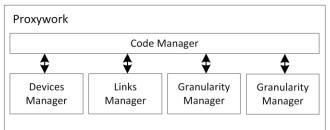
Figure 3 Proxywork software architecture
